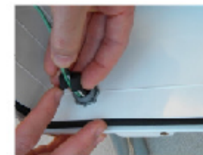
2) Open Vent Stop Plug and install over wire.
